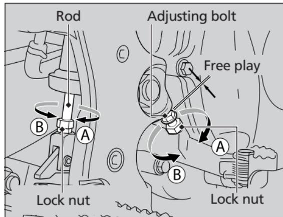
To adjust the rear brake pedal height:
