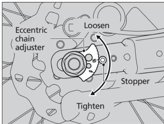
5. Turn the eccentric chain adjuster to a position with a larger number to reduce the free play of the chain or towards a smaller number to increase it.
