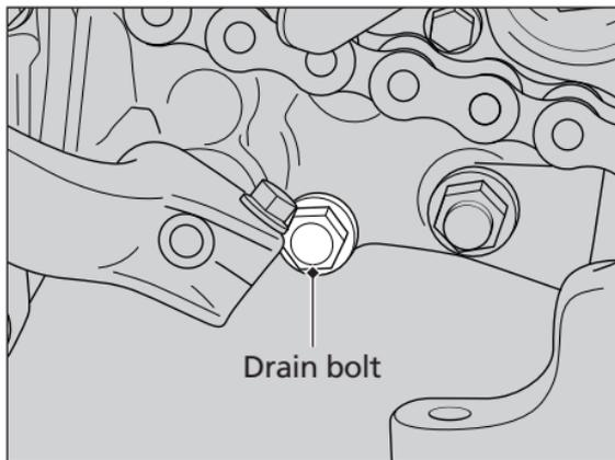
5. After the oil has drained completely, install the drain bolt with a new sealing washer. Tighten the drain bolt to the specified torque.
