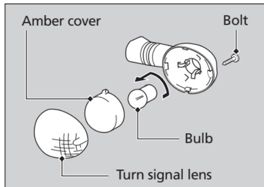
5. Install a new bulb and the rest of the parts in the reverse order of removal.
