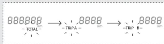
To reset "TRIP A" or "TRIP B", select the desired condition (accumulated mileage or ride time). Press and hold the (SET) button for more than 2 seconds.
