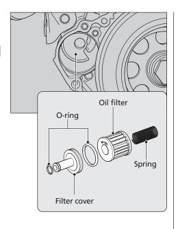
**14.** Install the new oil filter inside the crankcase, with its "OUT SIDE" mark facing out.
