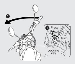
The steering lock is on the lower bridge of the front suspension.
