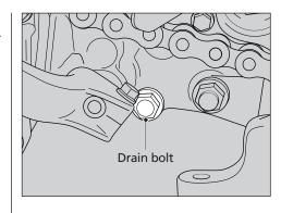
**5.** After the oil has drained completely, install the drain bolt with a new sealing washer. Tighten the drain bolt to the specified torque.
