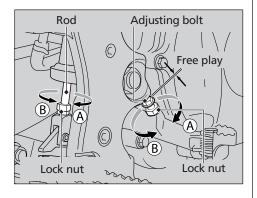
To adjust the rear brake pedal height:
