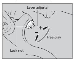
To increase free play, turn the adjuster counterclockwise, then tighten the lock nut securely.
