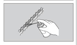
Avoid contact between the lubricant and brakes or tyres.
