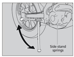
The stand is located on the right side of the motorcycle. It is used to support the motorcycle when it is parked. To activate it, use your foot to lower the stand until it is fully extended.
