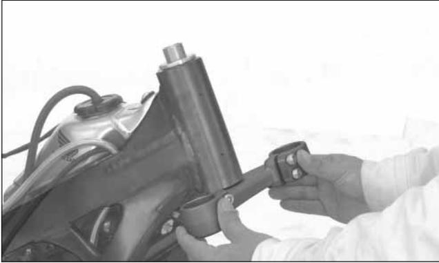
Turn the steering stem lock-to-lock 5 times to seat the bearings and retighten the adjusting nut to the specified torque.
