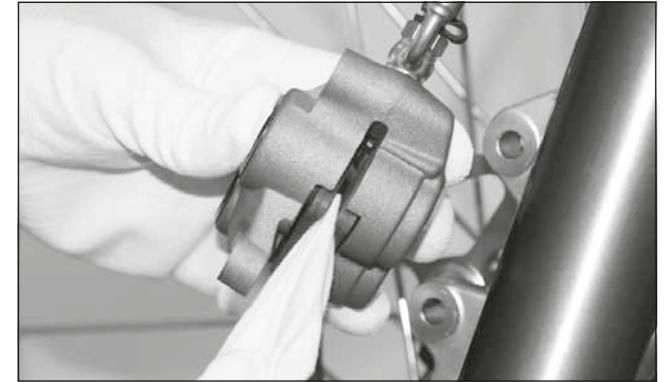
Push the pistons all the way in to allow installation of new brake pads.
