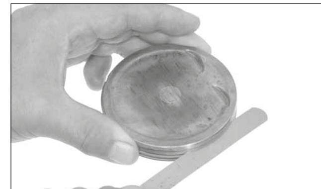
Temporarily install the piston rings to their proper position with the mark facing up. Measure the piston ring groove clearance with the rings pushed into the grooves.
