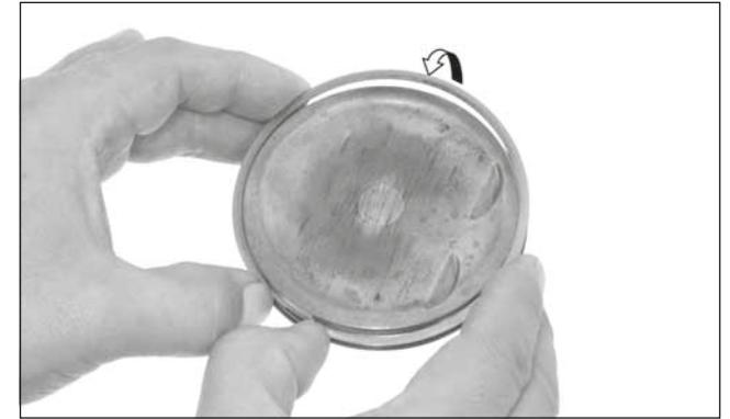
Spread the piston rings and remove them by lifting up at a point just opposite the gap.
