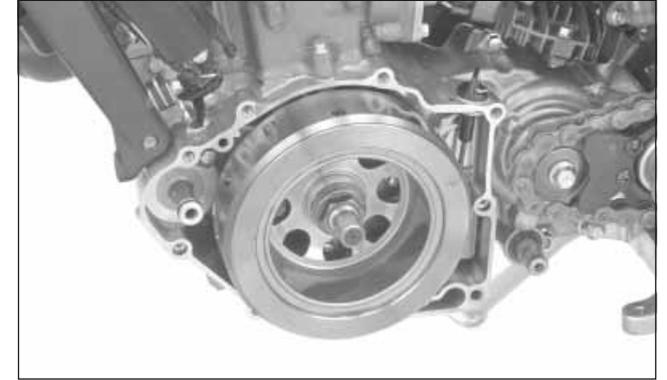
Hold the flywheel with flywheel holder, tighten the flywheel nut to the specified torque.
